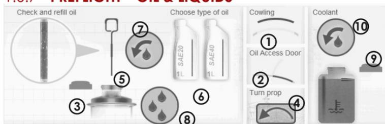
The **Oil & Liquids** window is the place to check and refill oil and coolant liquid.
