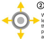
While holding down the left mouse button, drag the cursor up or down to push or pull the aircraft and left or right to turn the tow bar. Release the button to stop.
