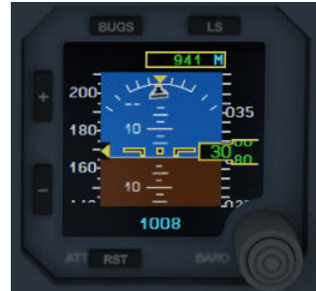
Integrated Standby Instruments System (ISIS)
